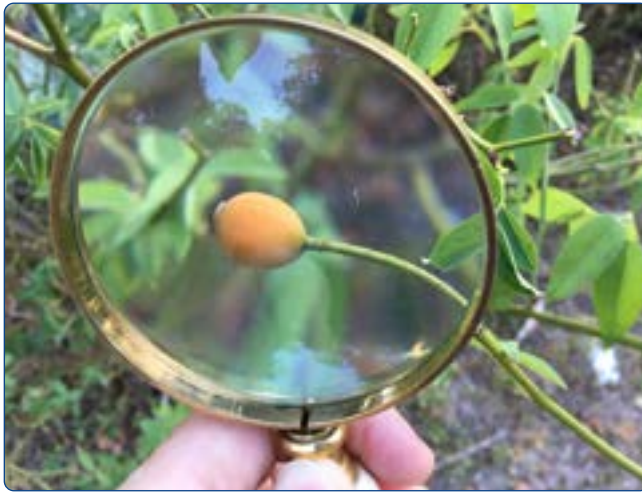
FIGURE 1.8. Magnifying glasses bend light so that objects appear to be larger than they really are. The magnification of a simple lens such as a magnifying glass is limited to about 2\times .
