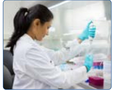
FIGURE 1.4. Experiments are one way that we obtain scientific facts. This picture shows a scientist using a micropipette, an instrument designed to transfer tiny, precisely measured volumes of liquid.
